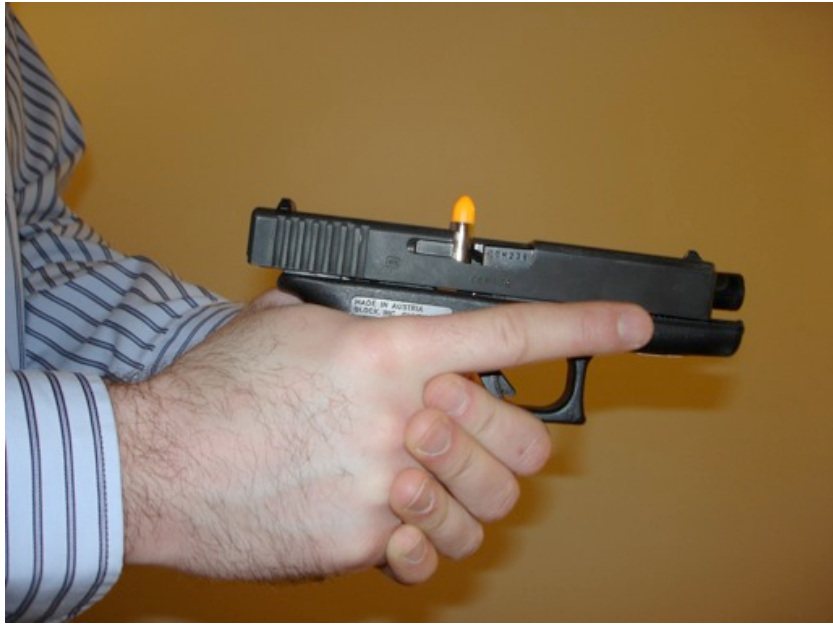
Type 2 malfunction - Stove Pipe
