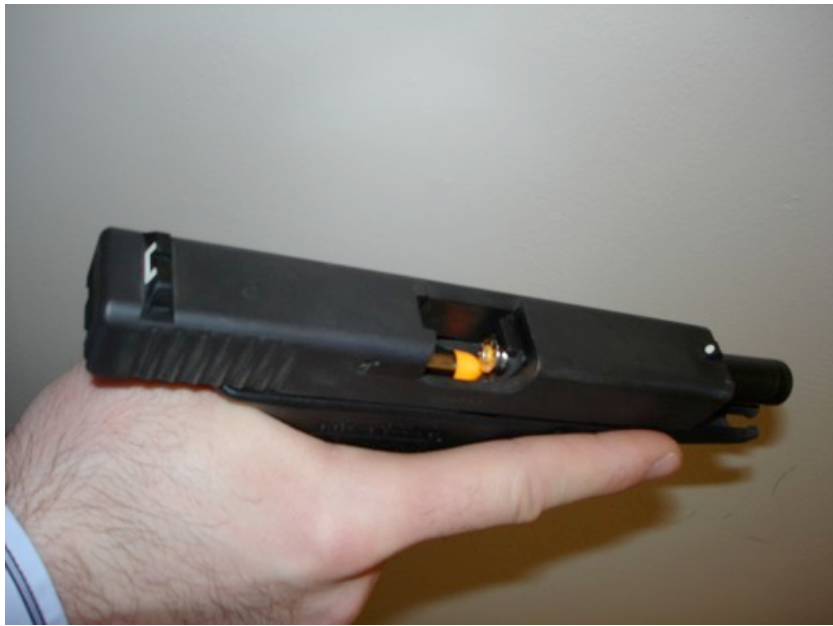
Type 3 malfunction - Double Feed
